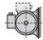
IM B7 IM 1061 foot wall mounted with feet on right-hand side when viewed from DE
